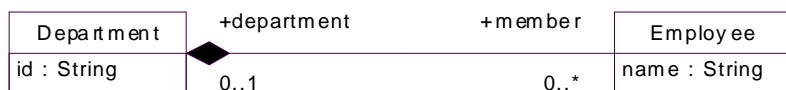
Figure 9.5 - Composite property serialized as XML elements, the opposite property is not serialized.
